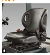
**ORS\* Seat with Suspension** \*ORS: Operator Restraint System
