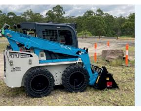
Like the 5SDK10, the 5SDK11 also offers vertical arm lift operation, helping to improve stability and easier dumping operability.
