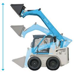
This design allows for optimal material handling. The bucket or attachment maintains the same distance from the machine making this ideal for truck loading of material or pallets and allows for better stability.
