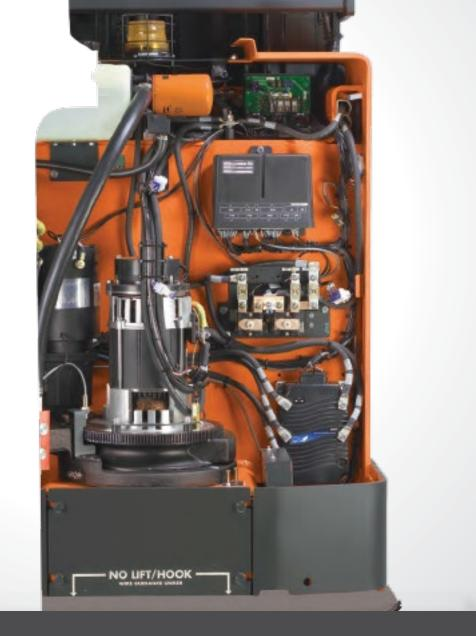
Automatic hydraulic staging of the mast cushions operation and reduces wear and tear for minimised maintenance. Regenerative braking and proportional plugging offer more responsive deceleration and vehicle control, extending the life of brushes and drive motors for reduced downtime.
